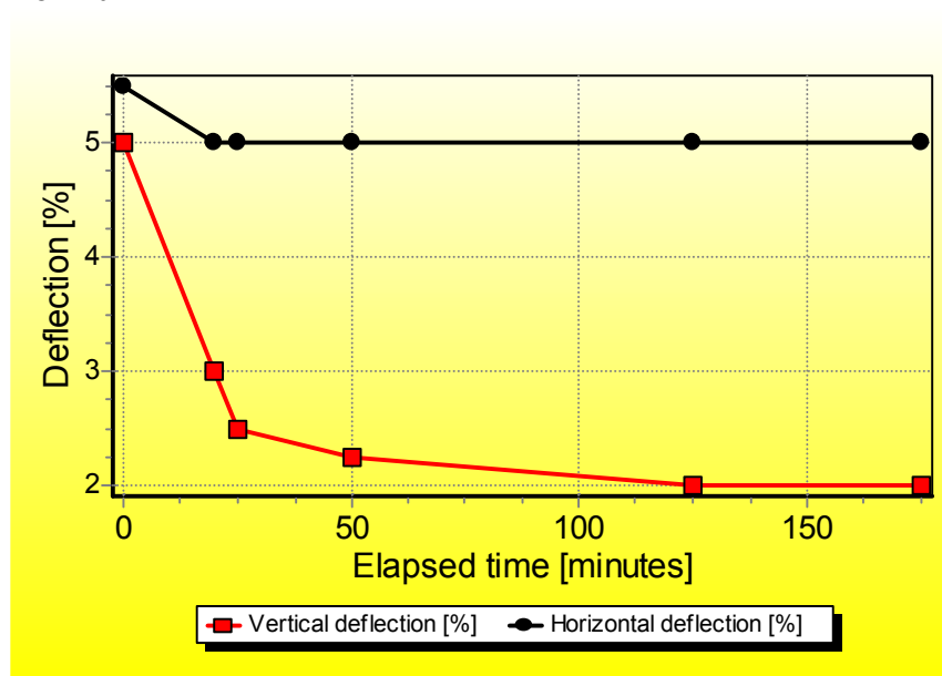
Figure 7: Re-rounding test on PE SDR26 pipes at the Wavin test site "Hammel" Denmark.
